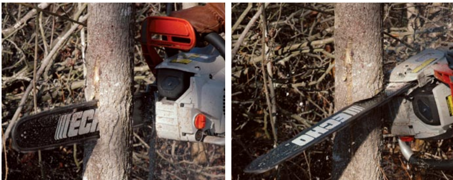
Larger trees tend to break instead of bend when half-cut, so the author uses a “T” cut. First, he makes a vertical plunge cut (left) at waist height slightly closer to the side of the tree in the direction of the fall. Then he makes a horizontal cut to form the “T” (right) on the side of the tree away from the planned direction of fall.
